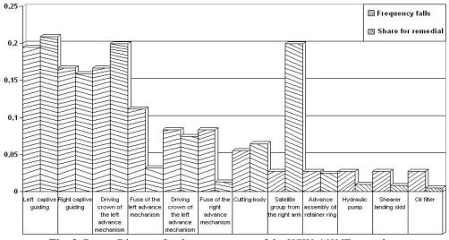
Fig. 3. Pareto Diagram for the components of the KSW-460NE type shearer
